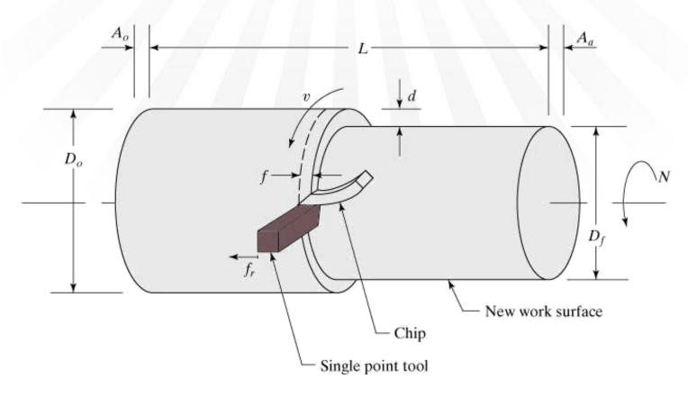
Key:  $D_o$  = staring diameter,  $D_f$  = final diameter, L = length, v = cutting speed, f = feed, d = depth of cut,  $f_r$  = feed rate, N = rotational speed, A = approach allowance, and  $A_o$  = overtravel allowance.
