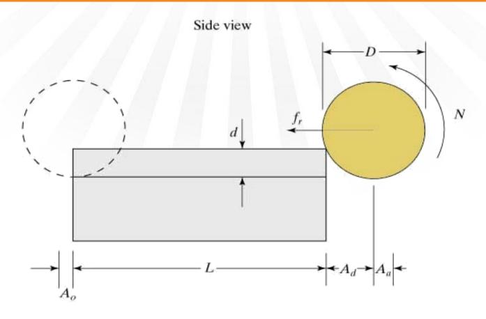
Key: D = cutter diameter, N = cutter rotational speed,  $f_r = \text{feed rate}$ , L = workpiece length, d = depth of cut,  $A_d = \text{distance to reach full depth}$ ,  $A_a = \text{approach allowance}$ , and  $A_o = \text{overtravel allowance}$ .
