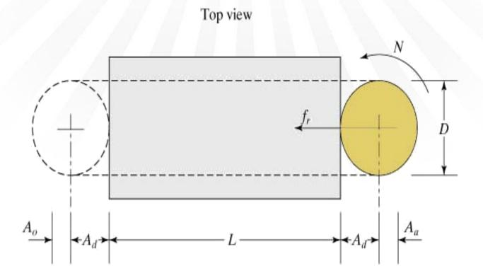
Key: D = cutter diameter, N = cutter rotational speed,  $f_r = \text{feed rate}$ , L = workpiece length,  $A_d = \text{allowance distance to reach full diameter (equal to overtravel distance)}$ ,  $A_a = \text{approach allowance}$ , and  $A_o = \text{overtravel allowance}$ .
