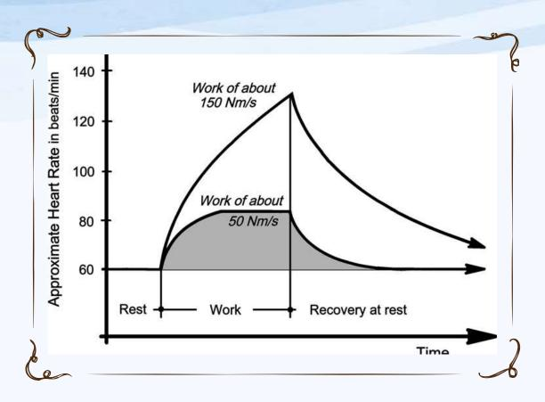
Heart rate at exhausting work and at steady state work
